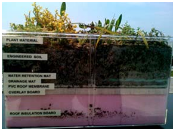
A green roof consists of seven layers, from the insulation board to the plant material.
