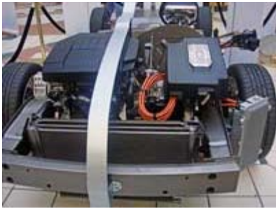
The Volt has a gas-powered generator (at right) and an electric motor (at left) that propels the car.
